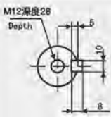
附帶鍵軸 Shaft with key
